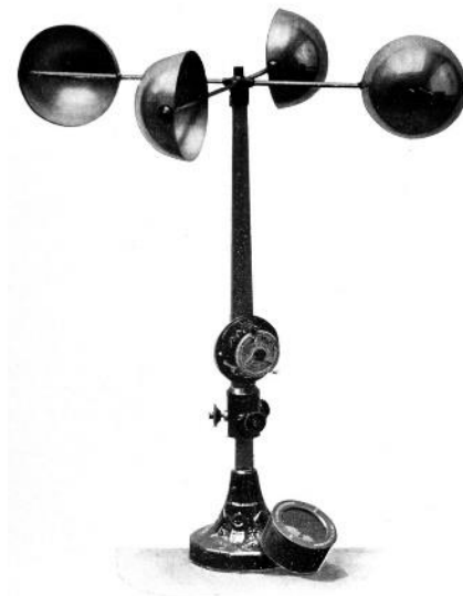
THE ROBINSON ANEMOMETER.
